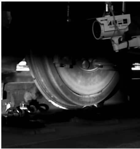
图 11 CRTS I 型轨道的碰撞情况 Fig. 11 Collision situation of CRTS I track
